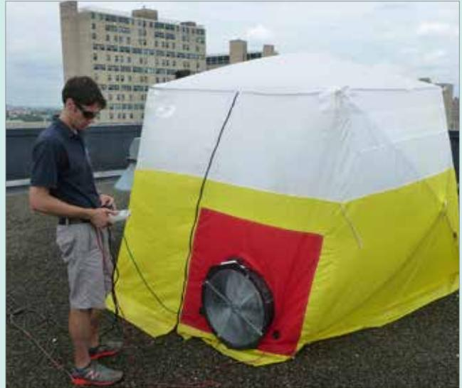
An auditor measures exhaust ventilation from roof top fans to determine if the line is over- or under-ventilated. Photo: Steven Winter Associates
