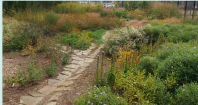
**Rain Gardens** are similar to bioswales but are more spread out and are located within a property rather than in a public thoroughfare. Like a bioswale, they include a stone layer, engineered soil, and planted area. The plants in this application must be able to tolerate both dry and wet conditions.
